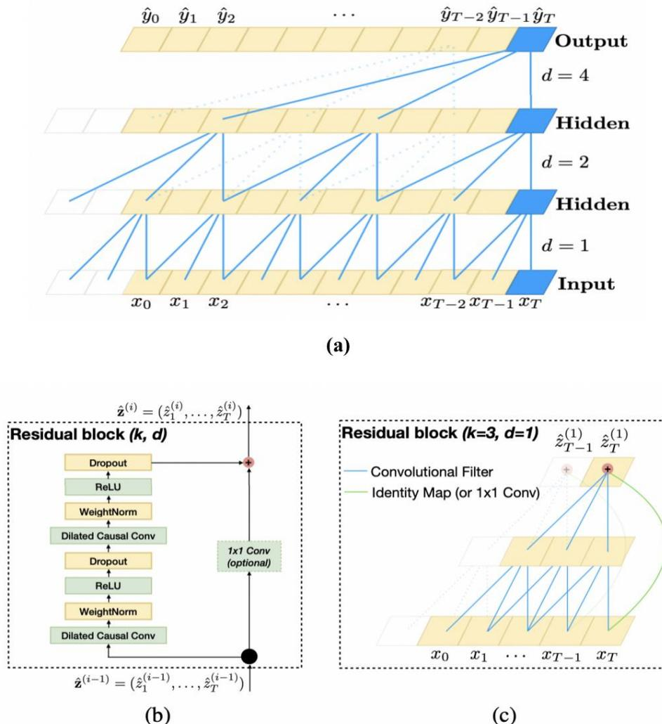
Figure 2. TCN Architectural . (a) All values in the input sequence can be sensed by the receptive field, and the expansion causal convolution, expansion factors  $d=1, 2, 4$ , and filter size  $k=3$ . (b) TCN residual block. When the remaining input and output dimensions are different,  $1 \times 1$  convolution kernel will be added (c) An example of residual connection in a TCN. The filter in the residual function is represented in blue, and the identification is mapped to green. [3]
